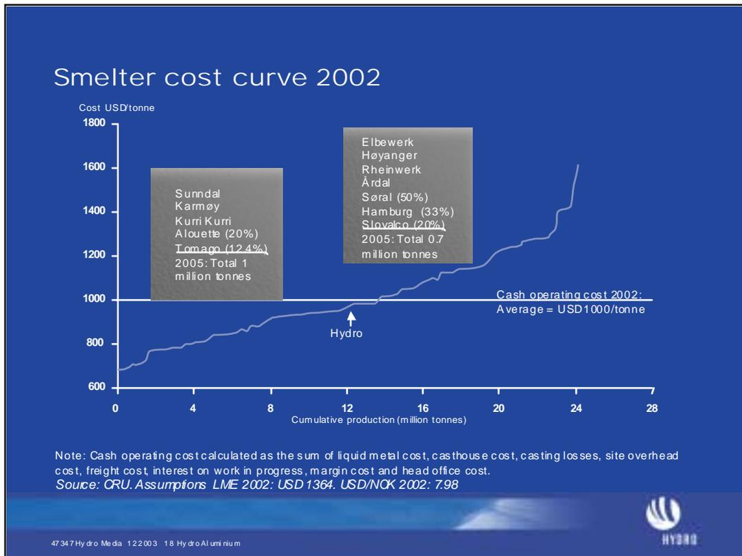
CRU Illustration: Cash operating cost on Y-axis. Accumulated global production X-axis.
